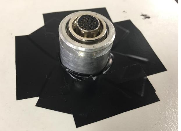
No direct electrical connection to Chassis & Body
